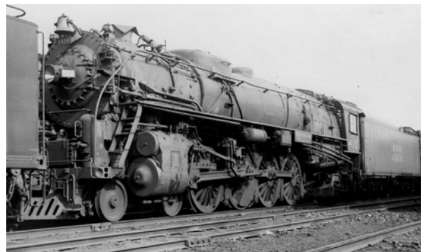
B&M Class R1c 4-8-2 No. 4110 at Boston, Mass., April 1947. The 'Calvin Coolidge' name plate is above the third and fourth drivers. (Photo by Dwight Smith)
